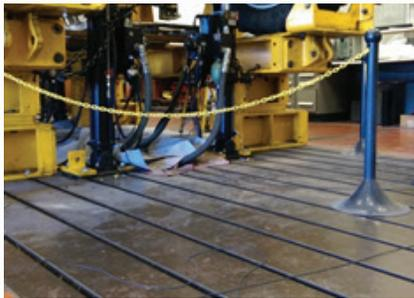
choosing the site location for the new shaker lab, a floor vibration study was conducted by ACS at the existing lab to evaluate vibration levels at the parking lot and outside perimeter of the client property. This data was used to evaluate the feasibility of extending the existing building into the parking lot, in order to house the new shaker lab.
